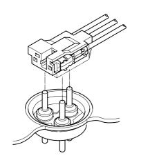
This three circuit connector is used to connect cluster pins (2.3 mm in diameter) to the leads of a motor hermetically sealed in a compressor of a refrigerator or a freezer.
